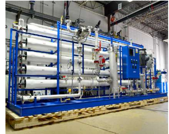
Industrial RO Plant
